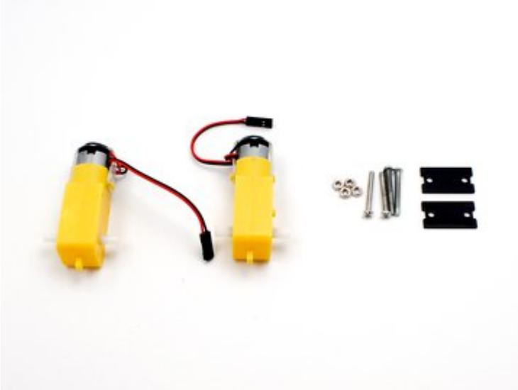
The metal panels go on the side with the red and black wires coming out.
