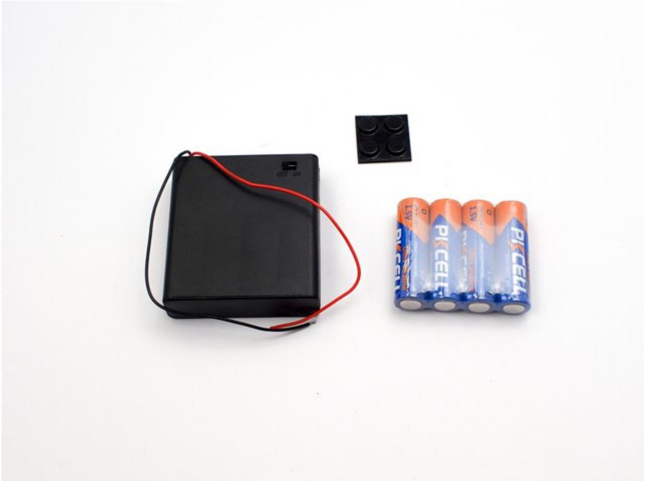
First, open each battery box, grab out the screw, insert your batteries, and then screw the boxes shut. **Oh, and make sure you have the boxes switched to the off position.** Now, take the 4 rubber bumpers and place them as shown in the picture below. Notice how the one bumper on the left side is not in the upper left corner. Important: don't throw away the leftover piece of bumper material, we are going to use that on the next step.
